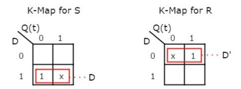
So, we got S = D & R = D' after simplifying. The **circuit diagram** of D flip-flop is shown in the following figure.
