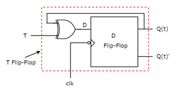
This circuit consists of D flip-flop and an Exclusive-OR gate. This Exclusive-OR gate produces an output, which is Ex-OR of T and Q t. So, the overall circuit has single input, T and two outputs Q t & Q t.'. Hence, it is a **T flip-flop**. Similarly, you can do other two conversions.
