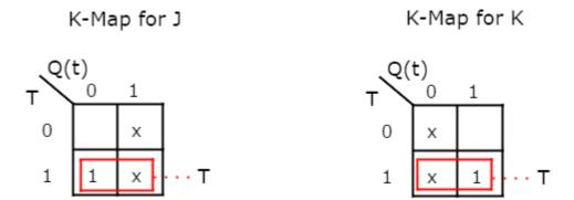
So, we got, J = T & K = T after simplifying. The **circuit diagram** of T flip-flop is shown in the following figure.
