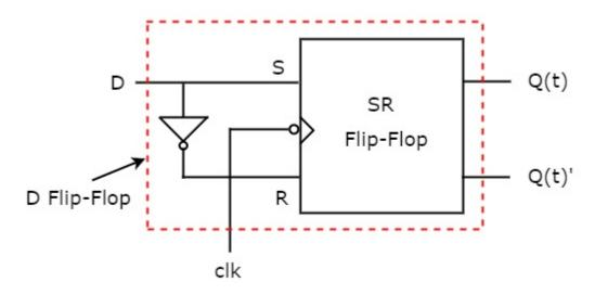
This circuit consists of SR flip-flop and an inverter. This inverter produces an output, which is complement of input, D. So, the overall circuit has single input, D and two outputs Q t & Q t '. Hence, it is a **D flip-flop**. Similarly, you can do other two conversions.
