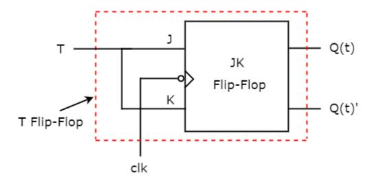
This circuit consists of JK flip-flop only. It doesn't require any other gates. Just connect the same input T to both J & K. So, the overall circuit has single input, T and two outputs Q t & Q t '. Hence, it is a **T**
