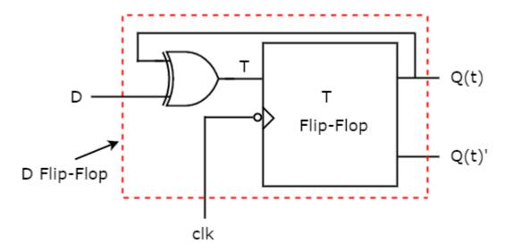
This circuit consists of T flip-flop and an Exclusive-OR gate. This Exclusive-OR gate produces an output, which is Ex-OR of D and Q t. So, the overall circuit has single input, D and two outputs Q t & Q t. Hence, it is a **D flip-flop**. Similarly, you can do other two conversions.
